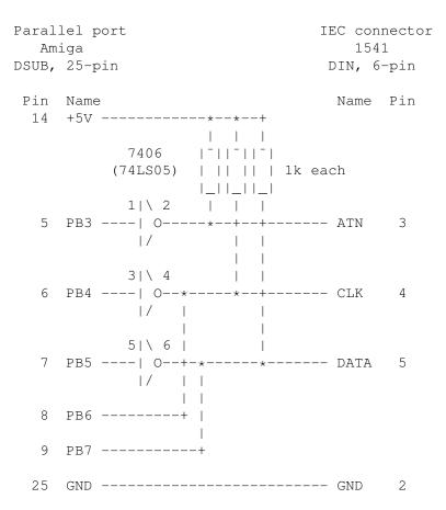
The 7406 (a 74LS05 will do as well) must be connected to +5V and GND of course. The trained technician will notice that this is the same circuit found inside the real C64.
